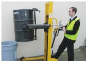
Raise drum using foot pump.
